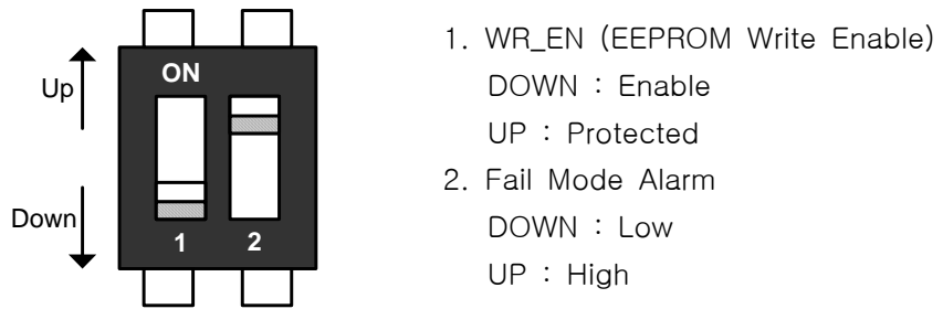
[Figure 6-6] DIP Switch Set-up in the CPU Module
