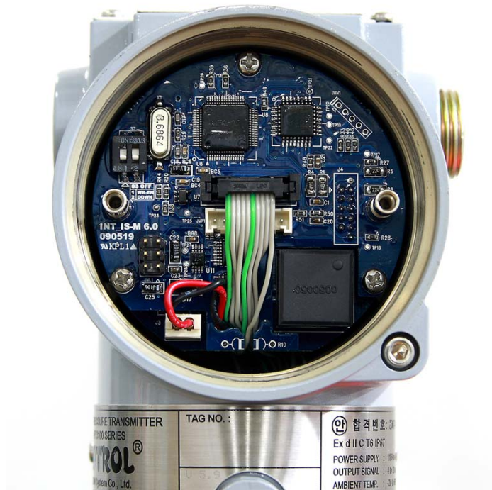
[Figure 7-1] Electronic circuit module
