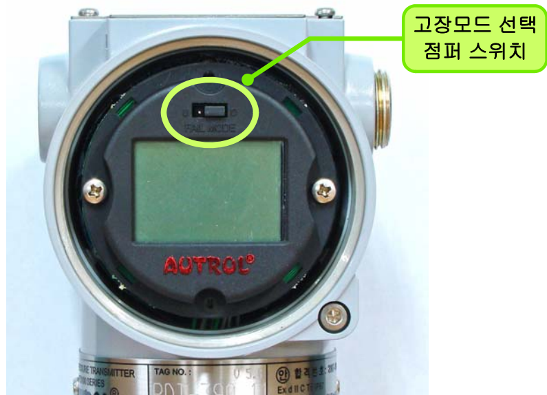
[Figure 6-7] Fail Mode Selection Jumper Switch in the CPU Module
