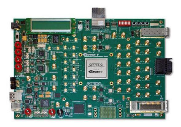
The Altera® Stratix® V GT Transceiver Signal Integrity (SI) Development Kit provides a platform for electrical compliance testing and interoperability analysis. The accessibility to multiple channels allows for real-world analysis as implemented in the system with transceiver channels available through SMA and popular backplane connectors. You can use this development kit to perform the following tasks:
