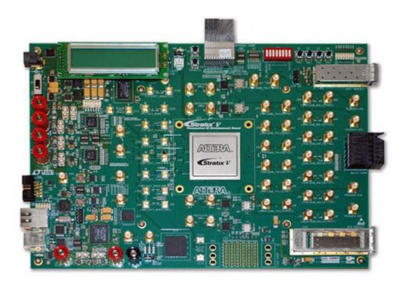
The Altera® Stratix® V GX Transceiver Signal Integrity (SI) Development Kit provides a platform for electrical compliance testing and interoperability analysis. The accessibility to multiple channels allows for real-world analysis as implemented in the system with transceiver channels available through SMA and popular backplane connectors. You can use this development kit to perform the following tasks:
