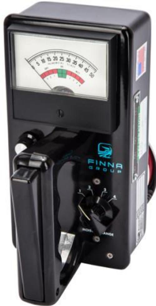
The Model A8 is similar to the T8, except that it has stainless steel buttons on the electrode. Designed for flat, curved, smooth, or rough surfaces such as cones or beams of yarn, rolls or stacks of cloth, rolls or stacks of paper or paperboard, carpets, tiles, etc. The electrode covers a 3 inch diameter area and the penetration is about  $\frac{3}{4}$  of an inch. Complete with Rechargeable Battery, Carrying Case and Operating Instructions Book.
