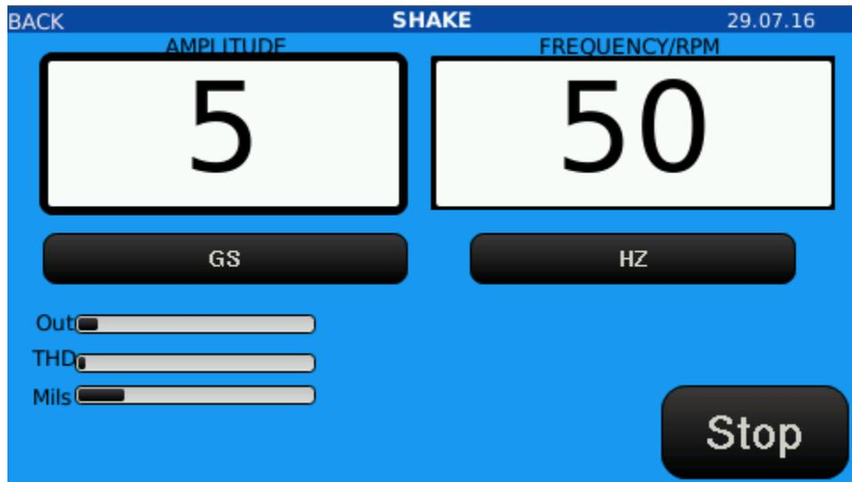
To manually test a transducer or equipment by only using variable frequency and amplitude:
