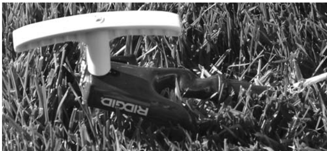
Figure 7 – Attaching Lead To Ground Stake
