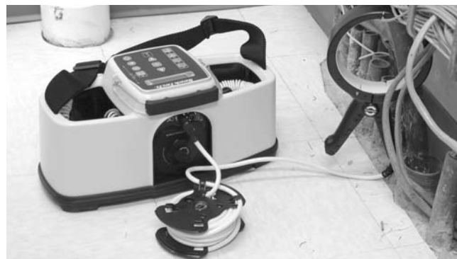
Figure 12 – Inductive Clamp Attached to a Conductor
