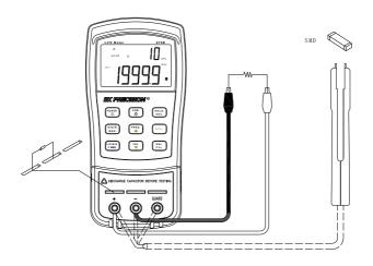
Figure 13 - Impedance Measurement Setup
