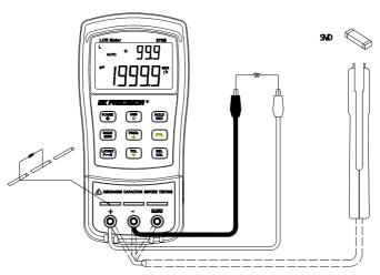
Figure 10 - Inductance Measurement Setup
