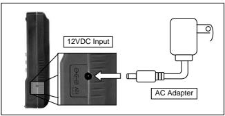
Figure 5 - Connecting AC Adapter to Meter
