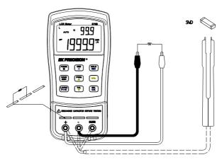
Figure 6 - Inserting Component to Inputs
