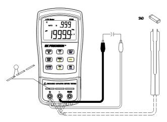
Figure 11 - Capacitance Measurement Setup
