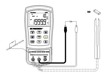
Figure 12 - Resistance Measurement Setup
