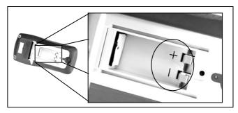
Figure 4 - Battery Compartment
