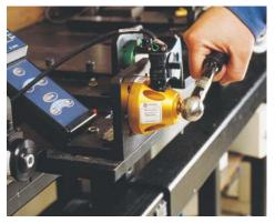
A BMX torque sensor is securely mounted for calibrating a torque wrench using a Mounting Bracket. Keeping the sensor in a stable position ensures the accuracy of the torque measurement during operation.
