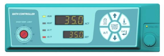
Step 2: Press to change the set point by using the button "UP/ DOWN ".
