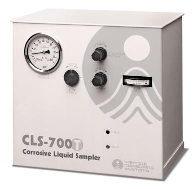
The CLS-700T corrosive liquid sampler is a compression sampler combined with a LiQuilaz® particle counter for effective measurement of particles in fluids contained in unpressurized vessels. The CLS-700T is ideally suited for testing effervescent chemicals. The system eliminates bubbles by pressurizing the sample and forcing the bubbles into solution.
