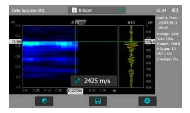
In this example the back wall is at 0.3m with a transmission time of 255  $\mu s$ . If the aim were to look for variation in thickness it would be reasonable to set the gate between 200  $\mu s$  and 300  $\mu s$ .
