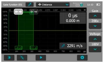
In order to find a suitable range, it is advisable to first carry out an automatic pulse velocity estimation and then to do a quick B-Scan to determine the range of the back wall.
