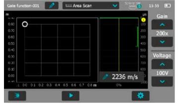
In the Distance and Pulse Velocity modes it is at the top of the measurement screen. In the Area Scan mode it is located in the A-Scan window at the right side of the screen.
