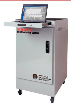
The AirSentry II Multi-point Monitoring System is the most advanced airborne molecular contamination (AMC) monitor available, utilizing sensitive and responsive ion mobility spectrometry to detect and characterize airborne molecular contamination from multiple locations within a cleanroom. The system features a 16- or 30-point manifold sampling system and an on-board computer with secure software and communications.
