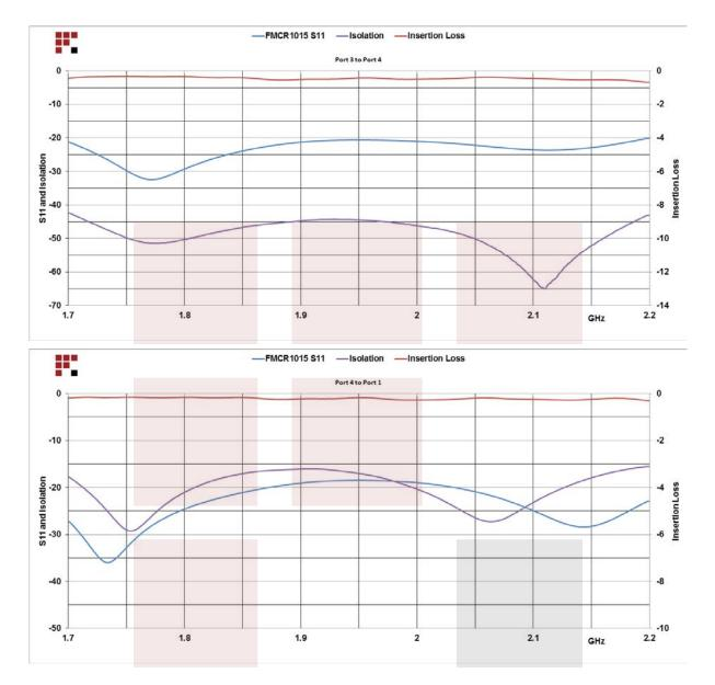
Dual Junction Circulator SMA Female With 40 dB Isolation From 1.7 GHz to 2.2 GHz Rated to 10 Watts from Fairview Microwave is in-stock and available to ship same-day. All of our RF/microwave products are available off-the-shelf from our ISO 9001:2008 certified facilities in Allen, Texas. Fairview Microwave is RF on-demand.
