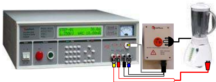
Figure 23: Tester Connected to an Appliance through a Corded Product Adapter
