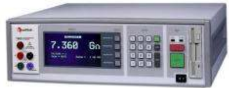
Figure 2: Typical Megohmmeter/IR Tester
