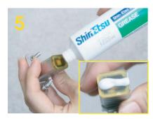
Put couplant onto surface of transducer as photo
