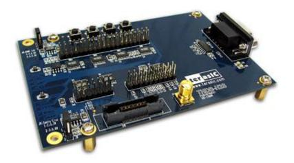
H2S (HSMC to Santa Cruz Card) is an adapter board for converting High Speed Mezzanine Card (HSMC) connector to Santa Cruz (SC) interface which allows users to use the SC interface boards on a board with a HSMC connector. Also, the source signals form the HSMC connector to the SC header on the H2S board pass through level shifters to adjust the logic level difference between the HSMC and SC interface board.
