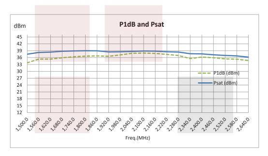
High Power Amplifier at 5 Watt P1dB Operating From 1.7 GHz to 2.5 GHz with 11 dB Gain and SMA from Fairview Microwave is in-stock and available to ship same-day. All of our RF/microwave products are available off-the-shelf from our ISO 9001:2008 certified facilities in Allen, Texas. Fairview Microwave is RF on-demand.
