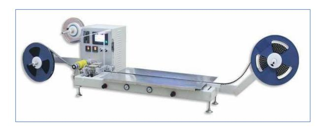
Tape & Reel Packing: Automatic seal, scroll and manual place the component.
