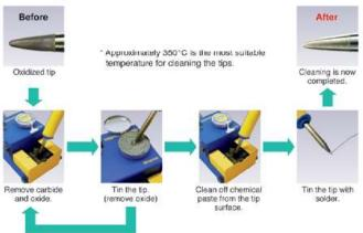
Repeat the process twice or more until oxide is completely removed.
