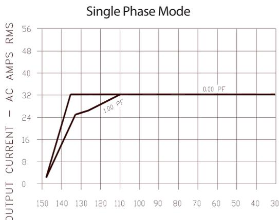
Short term overloads to 40A are permitted. Operating time before thermal shutdown or circuit breaker trip varies from seconds to severa; minutes depending upon line and temperature conditions.
