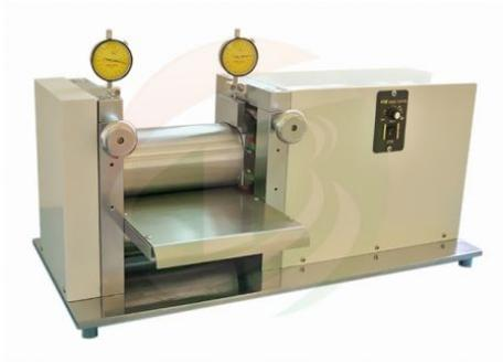
TOB-DR-200L Lab Roll Press Machine is a compact precision Electric Calender machine. It has dual rollers of 100mm dia. x 200mm width and dual grade micrometer.
