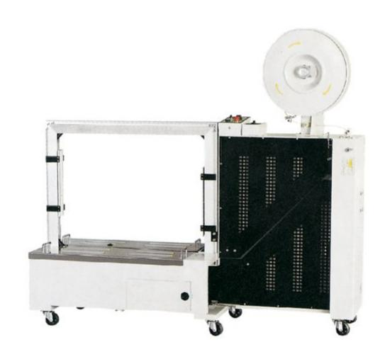
Electrical configuration: LG "PLC" control, France "TE", Japan "OMRON", "ZIK" electrical appliances, etc. It is suitable for large and heavy packing.
