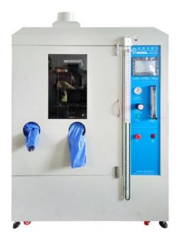
This instrument is mainly used to test the fire protection of insulation or coverings. This instrument is suitable for use in quality control, laboratory and other test sites where the flame resistance of the test material is required.
