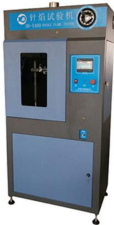
This instrument is mainly used to test electrical and electronic equipment and its components and components. It is also suitable for the test of solid electrical insulating materials or other combustible materials. It uses simulation technology to assess the fire risk of small flames caused by fault conditions inside the relevant equipment. It is suitable for electric wires, cable, plug, socket and other industries as well as quality control laboratories or research sites.
