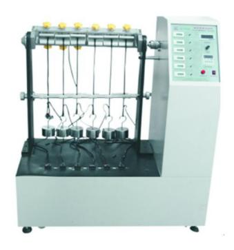
In line with IEC60884.1 (FIG21), GB2099.1, VDE0620.1 and other standards, it can be used in combination with our load machine to provide large voltage and current load for bending machine test. The instrument can be tested with or without load. The load connection mode is external connection, which can be connected to high-voltage and high-current load or low-voltage and high-current load mode.
