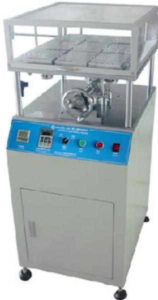
The main test USB interface durability plug and pull test.
