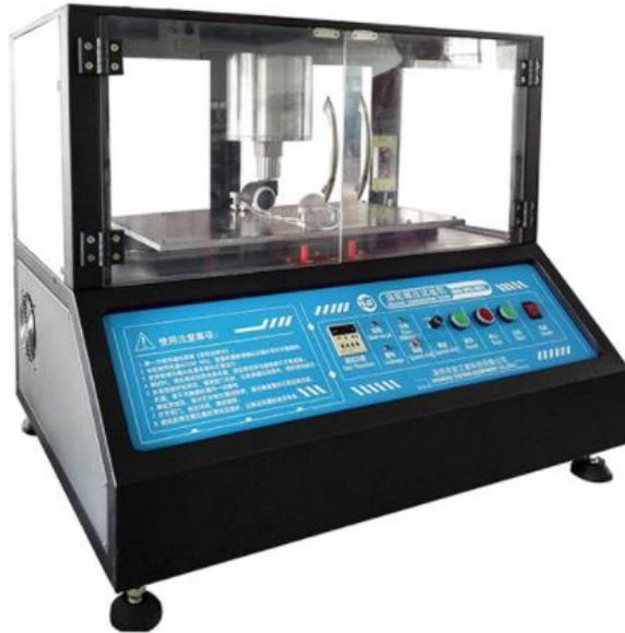
This instrument is mainly used to simulate the caster of the office seat repeatedly crushed on the wire to detect the crushing ability of the DC wire against the office chair wheel.
