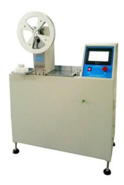
Designed according to the requirements of chapter 7.9 of APPLE's DC wire test standard 080-1276-k, it is used to detect the abrasion resistance of the outer layer of DC wire and has the function of judging defective products.
