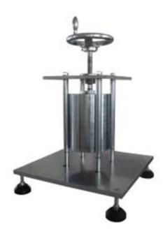
The HD-PCT plug compression test device is designed according to the relevant standards and is used for plug compression test to check the mechanical strength of the plug during compression.
