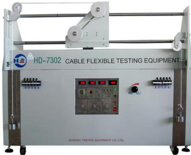
It is mainly used to test the special equipment for the alternating bending life test of PVC insulated wire and cable and rubber insulated wire and cable.
