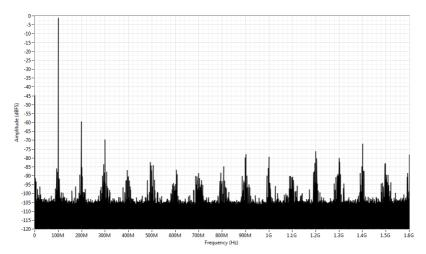
Figure 2. Single Tone Spectrum (Dual Channel Mode, 1.999 GHz, -1 dBFS, 3.2 kHz RBW), Measured
