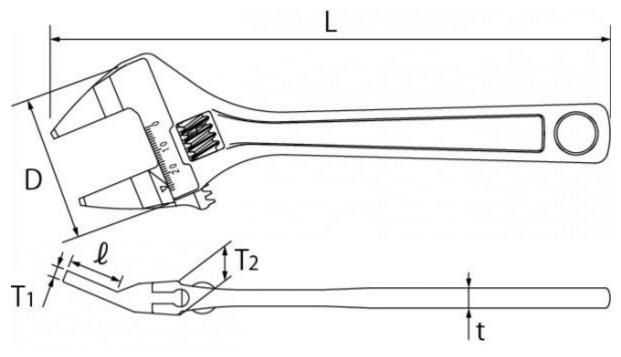
**backlash less knurl**2 knurls of Backrush less knurl holds jaw without tolerance. It can be used like open end spanner.
